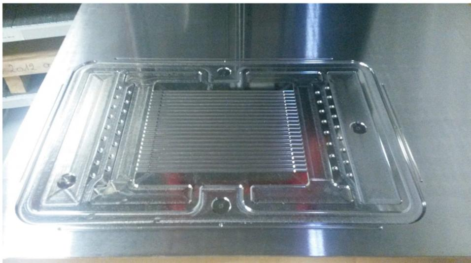
Figure 5. Die for hydroforming interconnects
