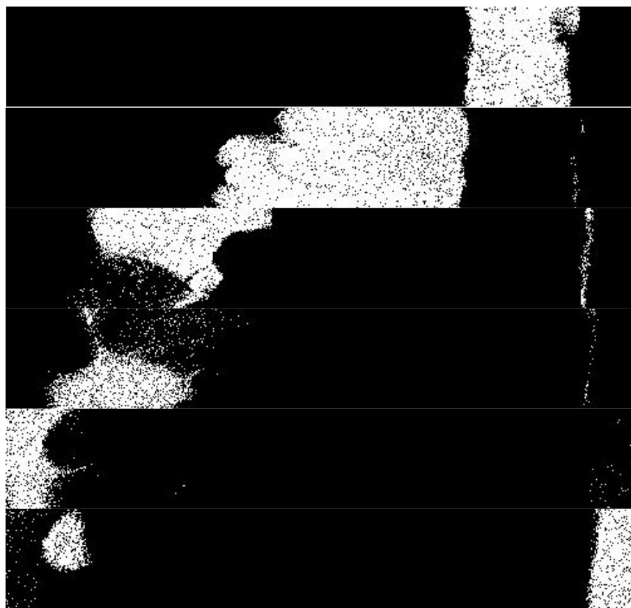
Figure 5. Trivariate diagram of Cr, MnO 2 and CoO fit coefficient maps of 02_72 h (Part I, Figure 3) showing six distinct regions: CrO x (ROI1), (Co,Cr)-spinel (ROI2), (Co,Mn,Cr)-spinel (ROI3-4), (Co,Mn)-spinel (ROI5) and steel substrate (ROI6).
