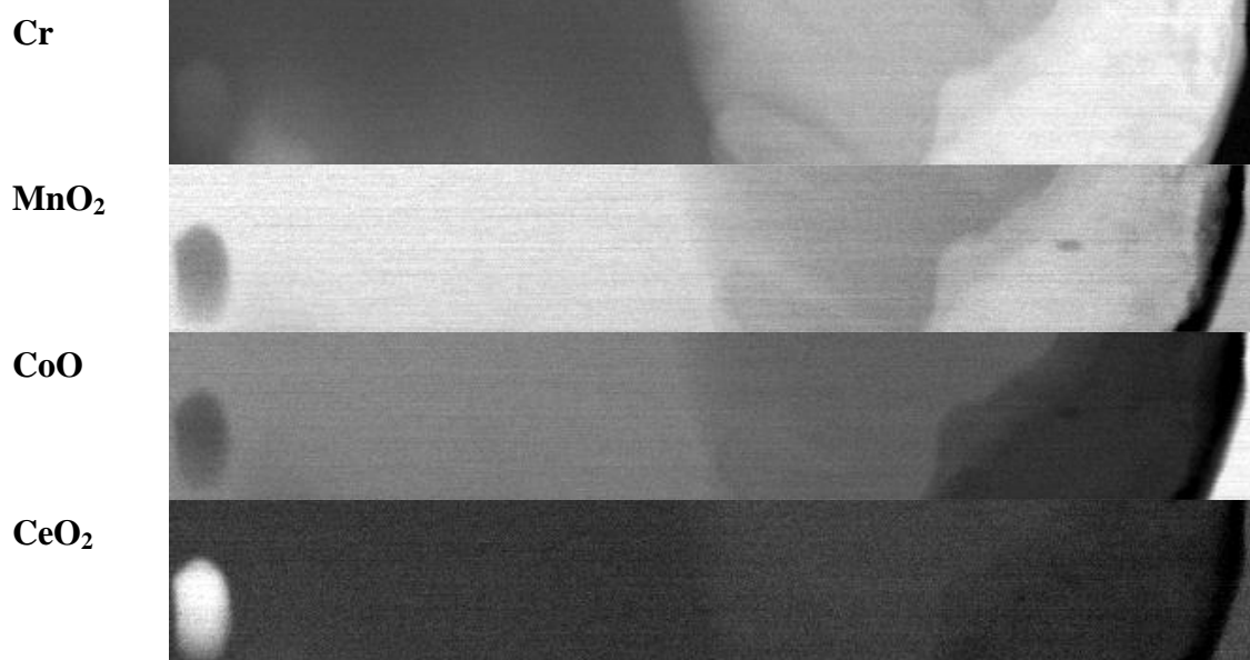
Figure 4. MLLS fit coefficient maps of Cr, MnO 2 , CoO and CeO 2 for the region from the steel substrate to the CeO 2 -layer after 168 h heat treatment. The arrow indicates Ce rich particles formed by redeposition of sputtered material from a larger CeO 2 -particle in the sample preparation process.
